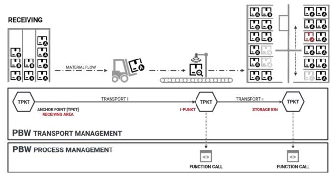
PBW transport control is used to perform all pending material movements in optimal order, i.e. usually as fast as possible and with a minimum number of transport steps. To solve this complex task, several strategies and the entire route network of the warehouse are stored in PBW.
