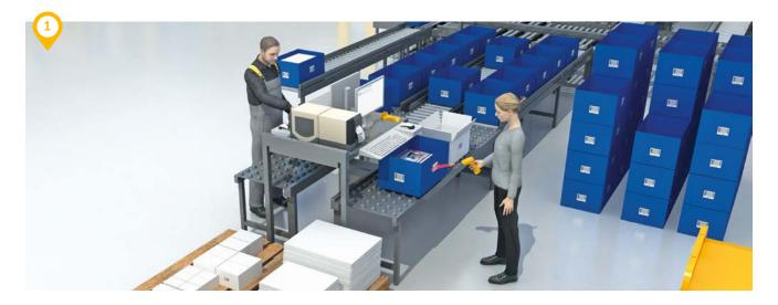
Automatic small parts warehouse (ASW) are always used when there are high performance requirements. The control and optimisation of the ASW is executed entirely by the Jungheinrich WMS. Both filling and order picking takes place in ASWs at upstream workstations. When order picking, using the **pick & pack** module, for example, enables the goods to be packed directly into a shipping unit during the picking process. As a result, two work steps are merged into one.
