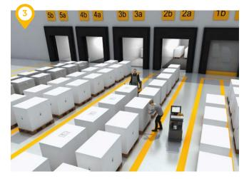
The **bypass module** ensures that just delivered goods for which a retrieval order already exists need not be stacked and are therefore immediately available for customer orders. The **cross-docking** throughput type is also supported by the Jungheinrich WMS.
