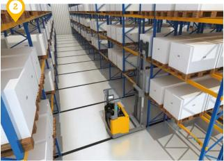
After collection, the stacking order can be created automatically or by the employee guided by the system. Then, in the course of the stacking, a mobile racking system, for example, is controlled by the Jungheinrich WMS and the corresponding destination aisle is opened. Other warehouse types such as drive-in or pushback racking, block storage warehouses, drive-through or cantilever-type racking can also be easily mapped in the Jungheinrich WMS.
