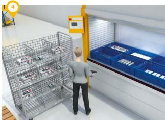
The **put-to-light module** increases process reliability by providing the employee with visual information for stack-ing.
