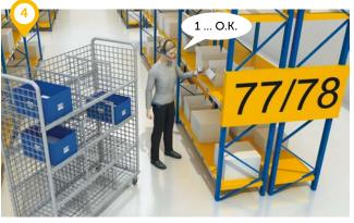
As an alternative to the wireless terminal, the employee can also be supported through **pick-by-voice** when order picking. The corresponding module ensures that your employees are able to keep their hands free for this. The result: Improved ergonomics with a simultaneously lower error rate.
