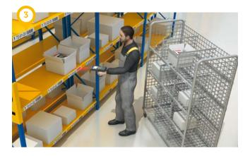
Are you using a **wireless terminal** for order picking? Then your employees receive all relevant information for retrieval in a clear, paperless form on the device – and in real time. The integrated scanner increases the efficiency of information acquisition.
