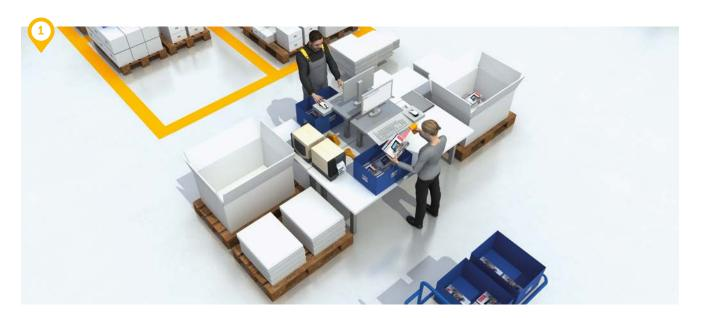
After removal, items from different warehouse areas are brought together at the consolidation area for the respective customer order. The **packing process** itself is, as a rule, controlled via a user dialog at a PC workstation. All the necessary documents such as the packing slips or shipping labels are printed in the course of the packing.
