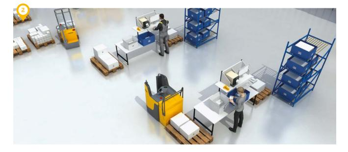
When processing production orders or during set formation, the Jungheinrich WMS controls the creation of a new item from two or more items. Following this, a new product label or other documents can then be printed by the Jungheinrich WMS. The **batches** of the individual components are saved when processing a production order and can be viewed at any time. This guarantees optimum traceability back to the individual component.
