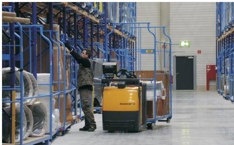
A Dedon worker takes a piece of furniture out of a storage rack and puts it on a furnibox, which is carried by an ECE 225 low-level order picker
