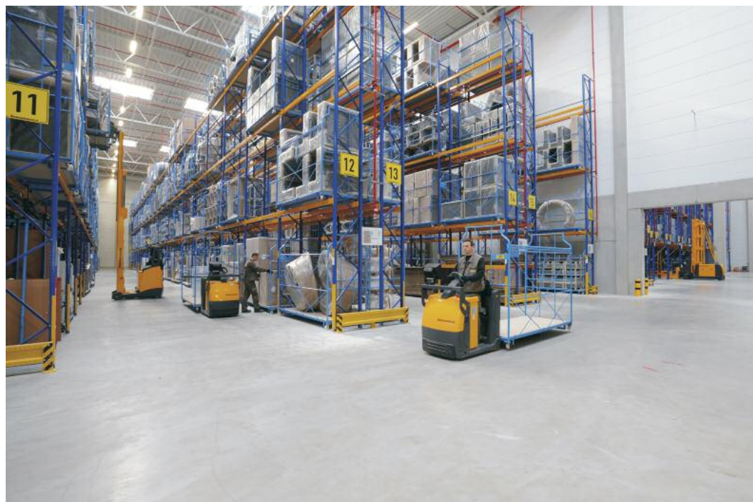
Jungheinrich has implemented the Dedon logistics center. The solution includes a Warehouse Management System, a WLAN system and forklift trucks with mobile data transmission terminals
