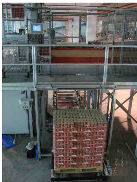
Handling equipment loaded for automatic depalletting Right: depalleting process
