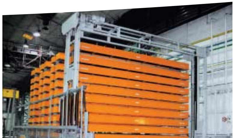
UNIPORTAL : Cassette Storage System with excellent space utilization. To handle small and medium amounts of material.
