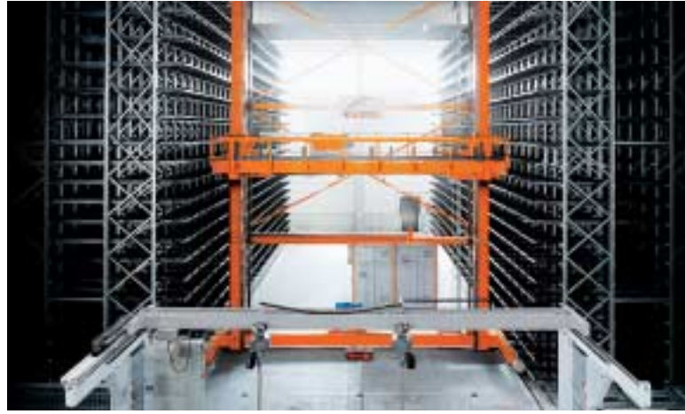
UNICOMPACT: Cost-effective Honeycomb Bar Storage System for medium to large storage volumes.
