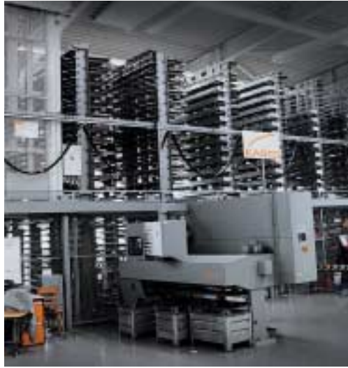
Sawing center for bar diameters up to 140 mm (5.5") at a manufacturer for brick making machinery.
