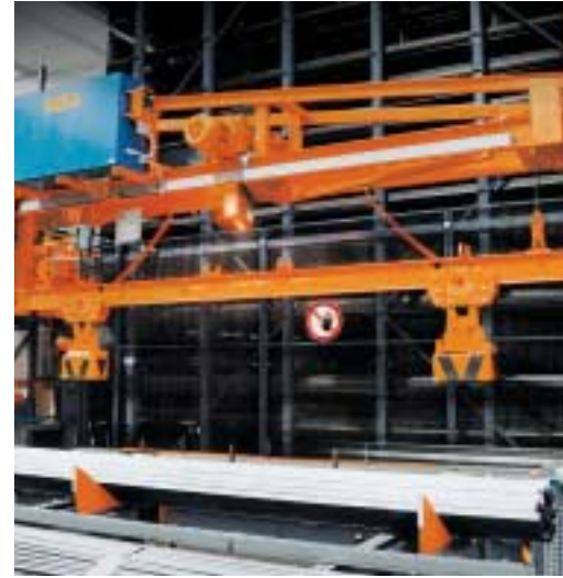
The commissioning unit allows ergonomic and fast material removal.
