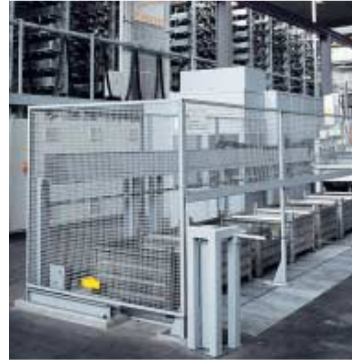
Sawing center with carbide circular saws for a sawing diameter of up to 260 mm (10.2") at a gear manufacturer.
