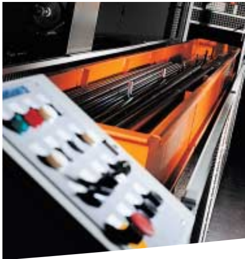
Move-out in longitudinal direction: Loading traverse deposits cassette onto a roller conveyor.
