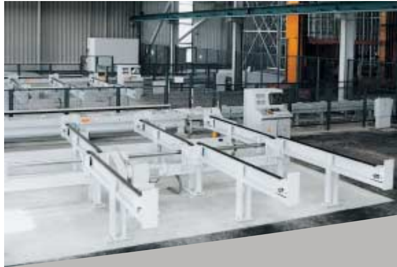
Order filling station with chain conveyor and a commissioning device.
