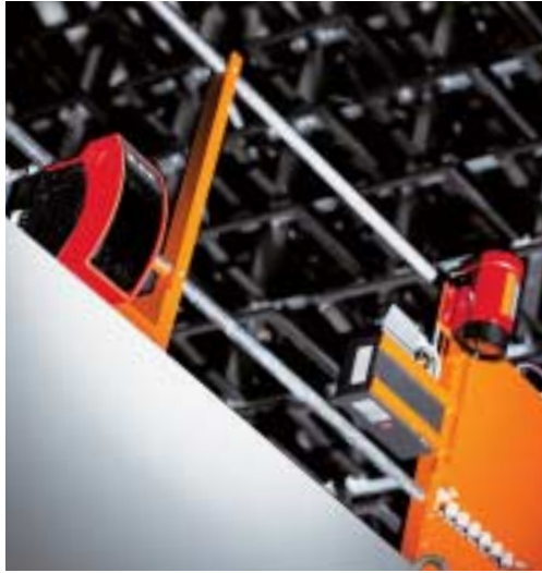
Infrared data transfer and laser axis ensure safe data transfer and interruption-free positioning of the operating gantry crane.
