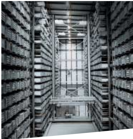
Commissioning system for plastic extrusions with 2 operating gantry cranes.
