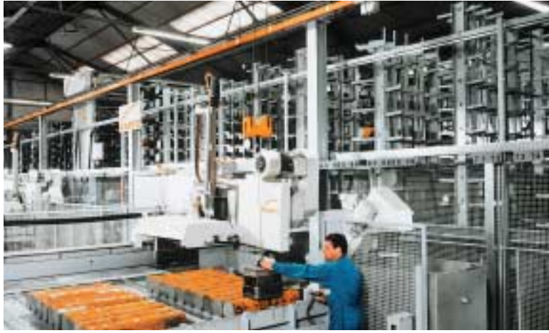
KASTOcenter: Combined Storage-Sawing-System. Especially universal with additional cassettes.
