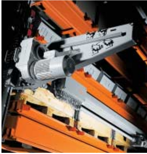
Robust and reliable: The chain hoist of the UNITOWER loading traverse.
