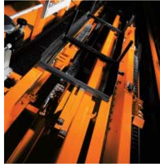
Operating gantry crane with pulling device for a reliable cassette transport.
