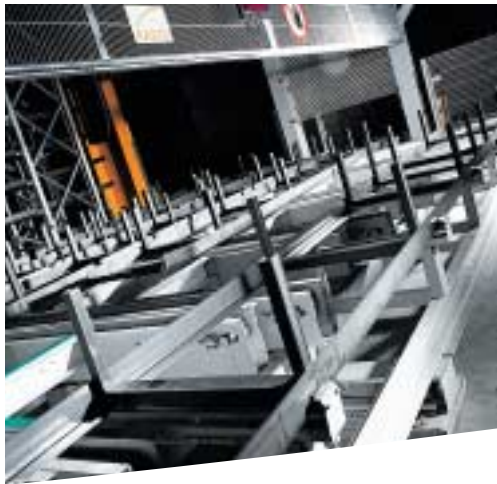
Continuous material flow: Carousel station with buffer locations.
