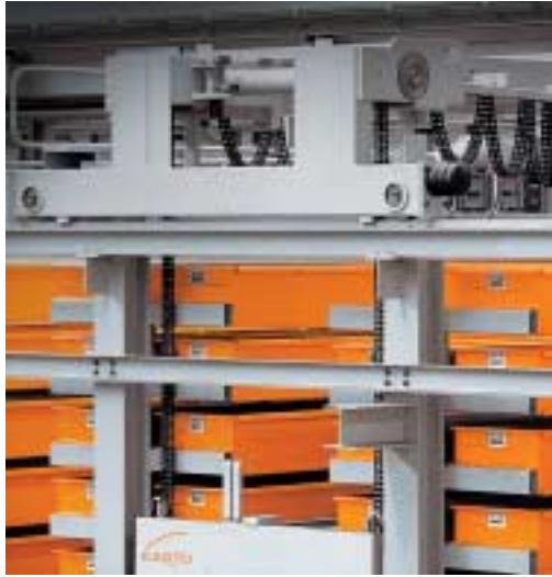
The chain hoist of the operating crane: Sturdy and durable.
