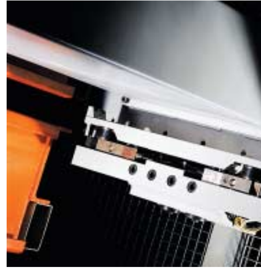
Weighing cells integrated into the cassette pick-up allow automatic inventory updates and constant inventory maintenance (option).
