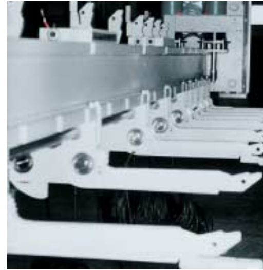
The KASTO loading traverse VarioPlus allows to pick up bars that are stored back to back.
