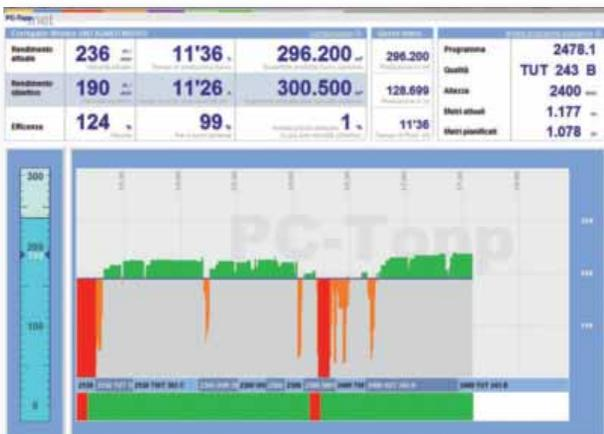
Corrugator Monitor: PC-ToppNET ensures the graphic visualization of the corrugator performances through the easy reading of the production speed trend, square meters produced and line efficiency. The graph, besides displaying, the average speed of the corrugator, also reports the graphics for the immediate performance reading, indicating for each combination the gap between the excellent speed and the speed which can be really reached in the production stage
